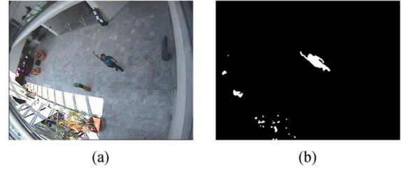
Fig. 3. Results of SOBS algorithm on sequence Walk1: (a) original frame; (b) computed moving object detection mask.
