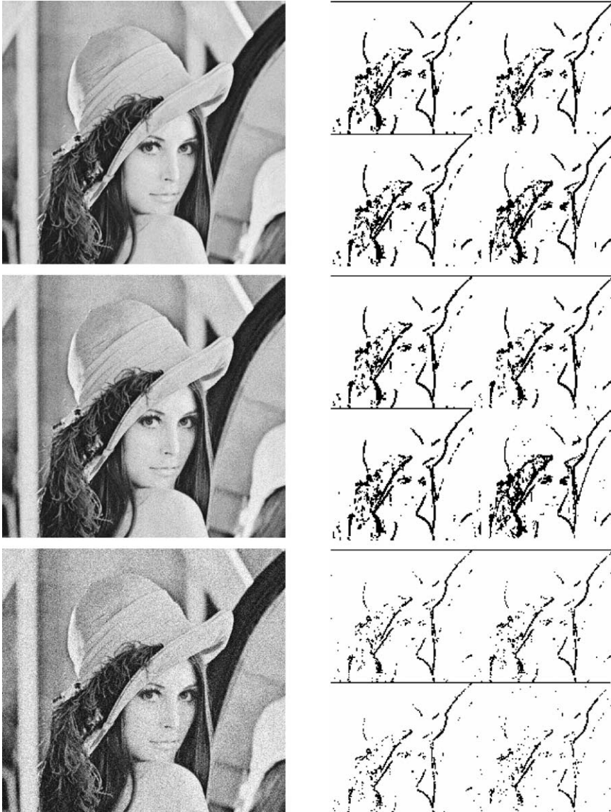
Fig. 5. In each row the original image corrupted by white noise ( \sigma = 3\% , 6\% , 12\% of the dynamic range) and the edge map obtained by the local operator Kirsh, Prewitt, Sobel and our method.
