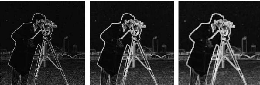
Fig. 3. Multi-scale gradient filtering with w = 3 , w = 5 , w = 9 . By column: G^3 , G^5 , G^9 .
